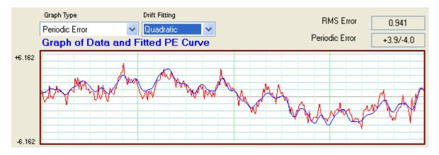
I then tried training the PEC on Gemini; unfortunately I only had enough clear sky to capture one and half cycles of data – not enough to perform any analysis. So here is just the raw data of the new block with PEC switched on in Gemini.
